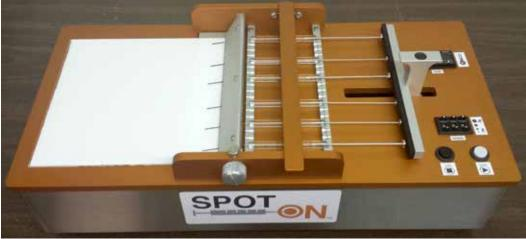
The **SpotOn™ TLC Sample Applicator** is a semi-automated device used to apply samples on Thin Layer Chromatography plates. The instrument eliminates the need for manual sample application and can be used to apply up to 18 samples at a time.
